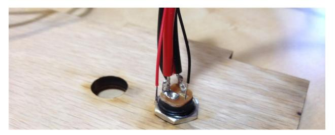
Note: I have an extra pair of wires soldered here. Don't worry about those. Just match the polarity to your Power supply. If the center pin is positive, be sure to match that to the red wire on your USB cable.
