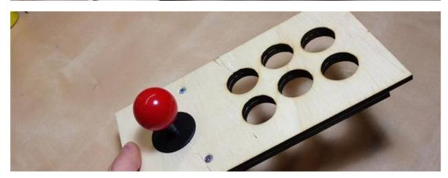
Insert the six arcade buttons in any color pattern you like. Tighten the plastic washers on the arcade buttons. This will clamp the two pieces together while the glue dries and ensure the two panels are aligned properly.
