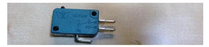
We will be using two of the three pins: Normally Open (N0) and Common (COM). These two tabs on the microswitch will be the circuit for each arcade button. When the button is pressed, the microswitch closes the contacts inside and the Raspberry Pi recognizes a button was initialized.
