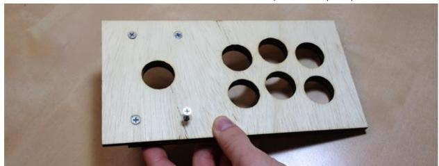
Flip the stack over and place the joystick over the four screws. Note the orientation; the five pins must face toward the button openings.
