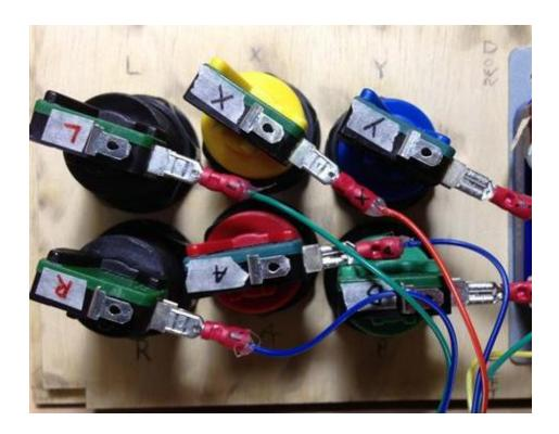
The directional (left, right, up, down ) micro switches on the joystick are easy in comparison. Remember those 5 pins are facing the buttons?
