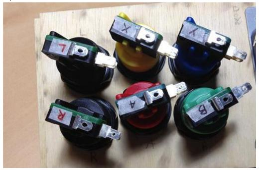
Plug the quick connect terminal end to the respective button/micro switches. Use the NO tabs (the middle tab).
