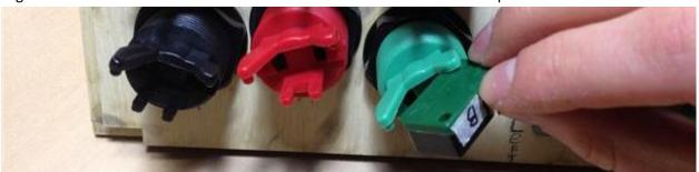
Push the other end of the micro switch into the button mount.
