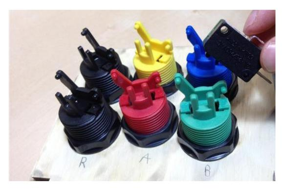
Align the lower hole on the micro switch and insert it into the short button pin.
