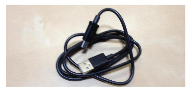
Cut the cable close to the regular USB "A" end.
